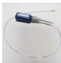
Dx-1 pH Probe and Dx-Transmitter
