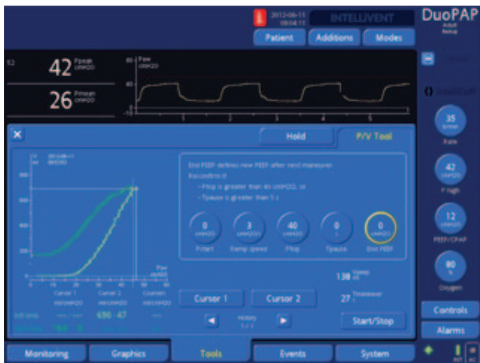
Figure 1. Example of the Pressure/Volume tool on the HAMILTON-G5 ventilator. Note the lower inflection point (setting of PEEP) is approximately 20-22cm/H 2 O for this ARDS patient.
