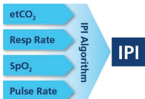
Figure 3. IPI combines four parameters into a single index.
