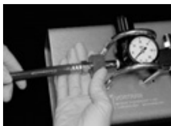
Figure B - Manifold is connected to source gas via a 20' tubing
