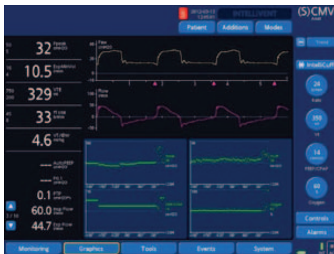
Automatic cuff pressure regulation over a 12 hour trend. (Pcuff in upper right trend panel). Brief period of increased cuff pressure is due to coughing episode (Peak Pressures in upper left hand panel).
