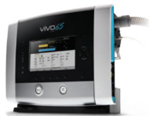
Figure 2. Vivo 65. The eSync triggering algorithm calculates the patient diaphragmatic flow during inspiration using Joules of energy. The minimal trigger of the Vivo 65 is 0.2 L/sec 2 compared to 1-2 L/min for the average home ventilator.
