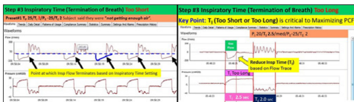
Figure 7. Step #3: Evaluation of the inspiratory time setting illustrating instances in which the Inspiratory time was set too short (left hand panel) vs inspiratory time set too long (right hand panel). On the left hand panel the dotted horizontal blue line in the flow trace is drawn at the zero flow line. In this subject the inspiratory flow is decaying towards zero as the lung fills, but the breath is cut short (black arrows) by the inspiratory time setting. This subject was very tall with a large vital capacity and needed a longer inspiratory time to complete the breath. On the right hand panel the green rectangle represents the time necessary for the subject to complete their natural inspiratory breath at an inspiratory time of approximately 1.1 sec, however the pink rectangle indicates that the actual inspiratory time setting was 2.5 sec which was too long.
