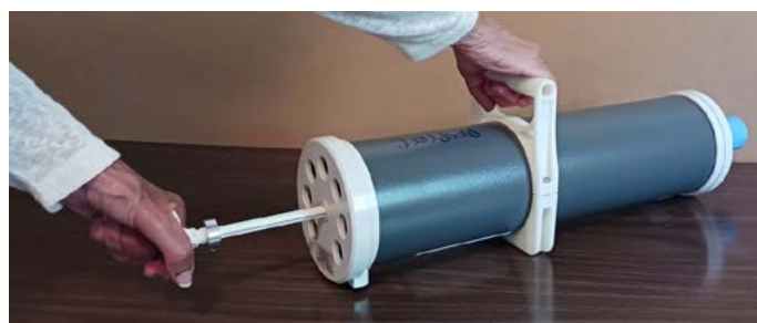
Figure 2. The syringe handle provides a firm anchor for holding the syringe when performing calibration maneuvers.
