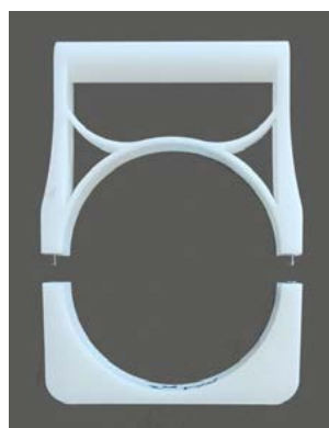
Figure 1. The syringe handle is secured to the body of the calibration syringe.
